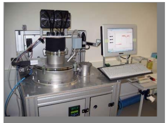
Picture: Nye's ASTM E-595 Outgassing Test Rig
