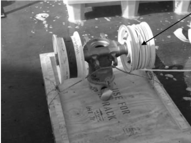
Figure 7 – NLG wash test rig
