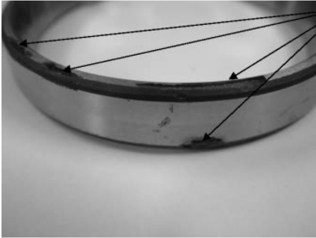
Figure 11 – Salt water immersion MIL-PRF-81322
