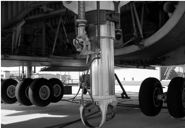
Figure 3 – C-5 landing gear
