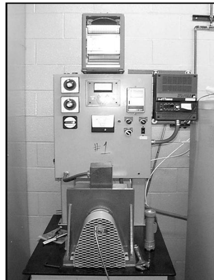
Figure 2 – High speed bearing test rig (Ref. 5)
