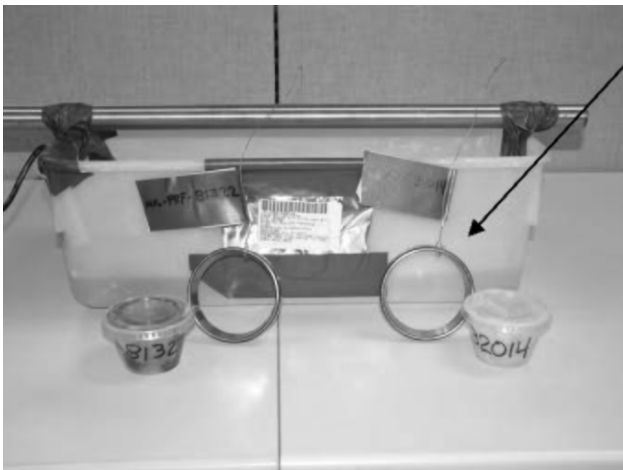
Figure 9 – Salt water immersion test rig
